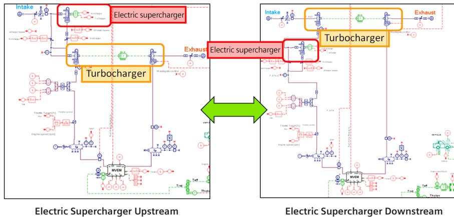
Comparison between electric supercharger upstream and downstream positioning.
