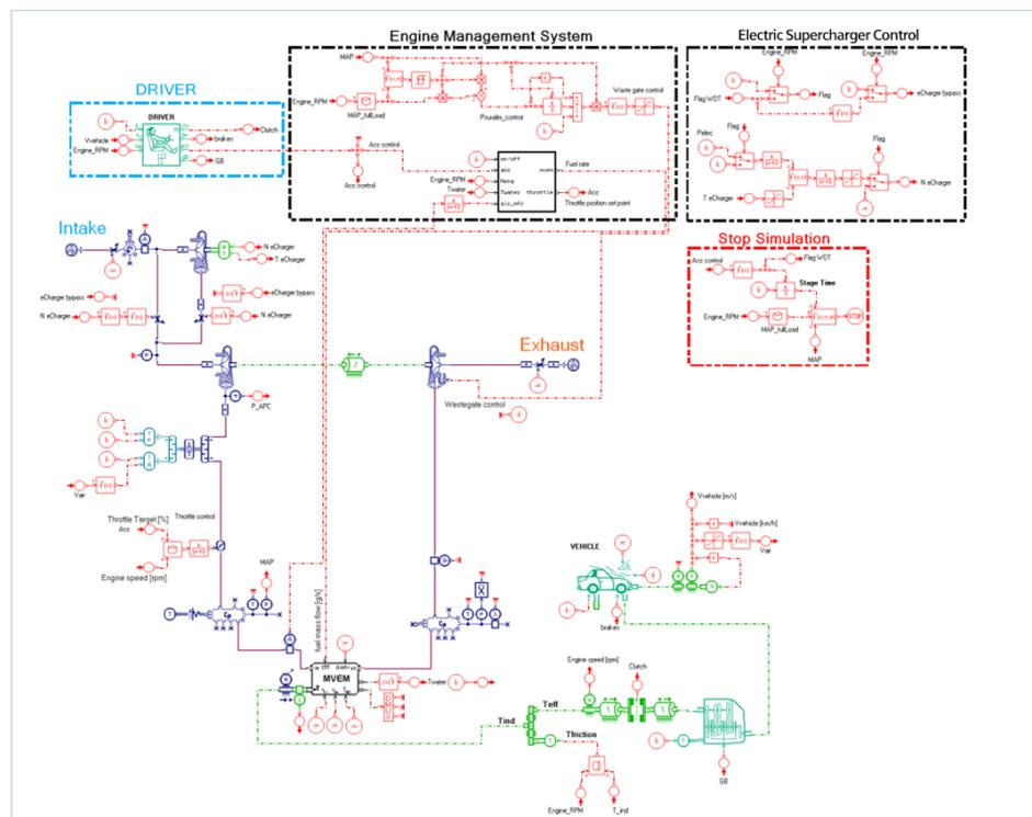
The LMS Imagine.Lab Amesim simulator model of the electric supercharger vehicle.
